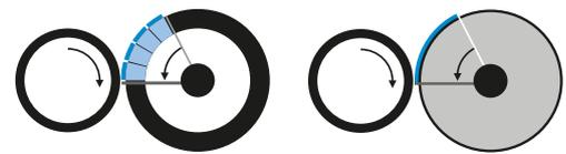
Marking wheel with segments    Marking wheel with solid engraving
